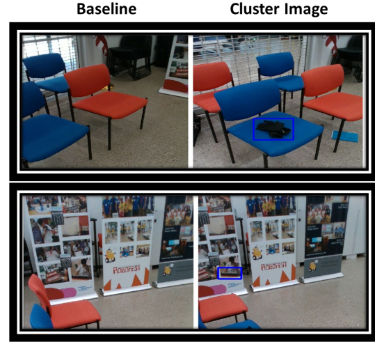
Figure 4. Example merged images processed by the VLM to search for change in the lecture space. (top) A “small item” has been introduced. (bottom) A keyboard in a hanging poster is flagged as “electronics”
